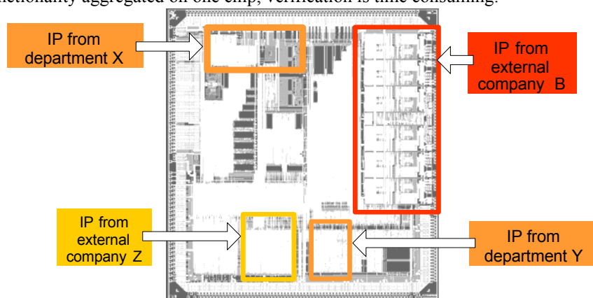
Figure 1 IPs Integrated on a System on Chip
